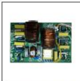
⑤ Power filter board
